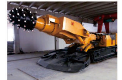
掘进机 Tunnel boring machine
